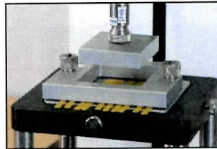
Pasta Firmness and Stickiness Fixture Measures the firmness and stickiness of uncooked pasta. Fixture Base Table required. TA-PFS
