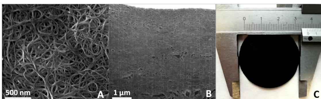
**Fig. 1.** The morphology of oxidized SWCNT membrane observed from (A) top and (B) cross-section. (C) Optical image of as-prepared freestanding BP prepared from oxidized SWCNT.
