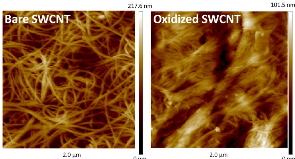
Fig. 2. Morphology of BP made of bare and oxidized SWCNT obtained by AFM.
