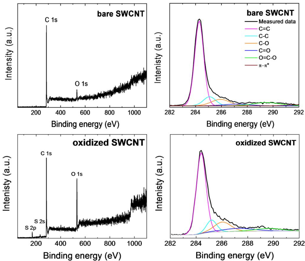
**Fig. 4.** XPS survey spectra and high-resolution spectra of C1s region of bare and oxidized SWCNT.
