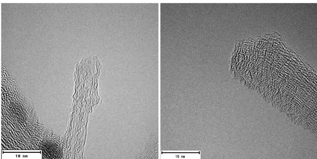
**Fig. 3.** HR-TEM image of agglomerated oxidized SWCNT end tips showing highly that oxidation damage mainly nanotube end tips.
