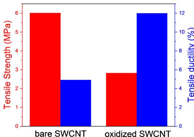
Fig. 5. Tensile strength and ductility of BP prepared from bare and oxidized SWCNT.
