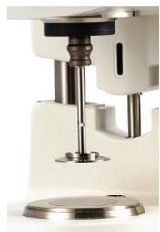
Choice of cone spindles and plate spindles accommodates various sample types. Plate spindles can be used for highly-filled or very viscous samples.
